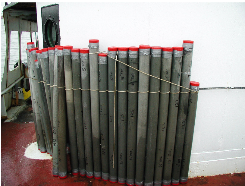
Photo shows cores labeled and stored vertically on board the vibracore drilling vessel.
