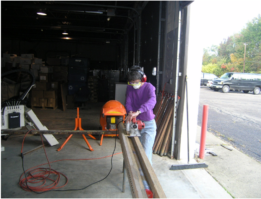
Photo shows proper placement of saw on jig and operator with required protective gear.
