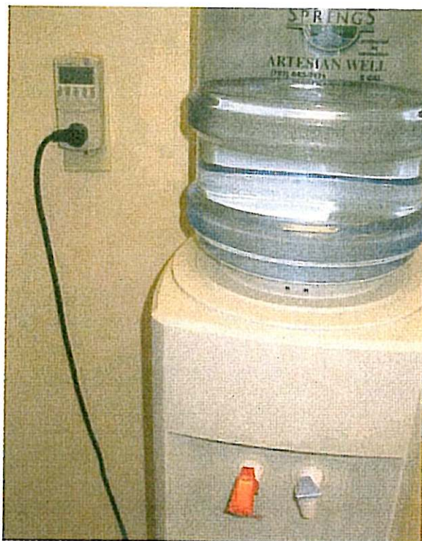
Figure 13. Hot/cold drinking water dispenser (power meter reads 520 Watts)
