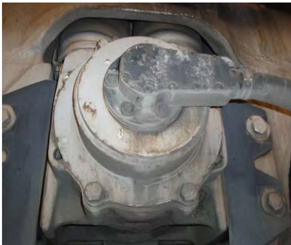
Typical end of Axle Mounted Axle Drives (speed sensor)
