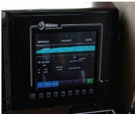
Typical Central Display Unit (CDU)
