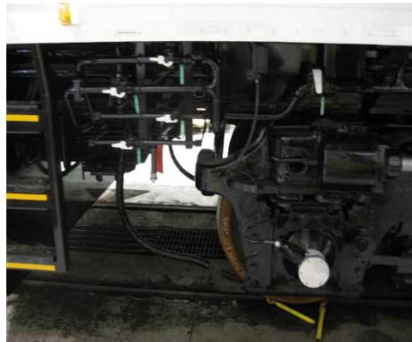
Typical end of Axle Mounted Axle Drives (speed sensor)
