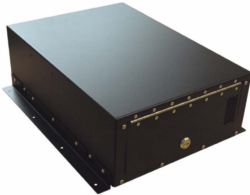
Figure 4 - Typical DVR with Locked Enclosure
