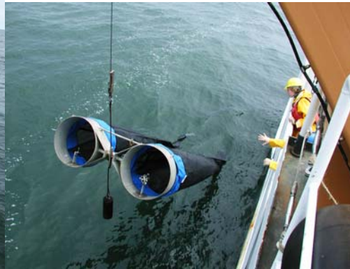
Bongo net 0.70m paired net 505 \mu m mesh Towed obliquely at 2-3 knots Max depth 100m (54 fathoms) Weight 200 lbs
