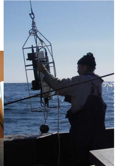
CTD Lowered vertically with a max depth of 500m (274 fathoms) Weight 70 -100 lbs.
