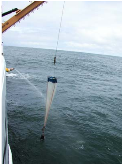
Vertical net 0.5m diameter ring net 202 \mu m mesh Towed vertically Max depth 100m (54 fathoms) Weight 70 lbs
