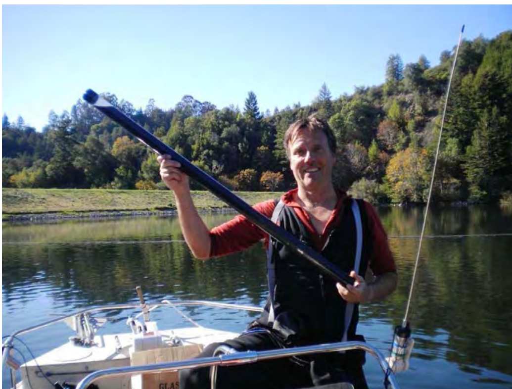
Photo 2: Sludge sample collected in 4' x 2" acetate liner.
