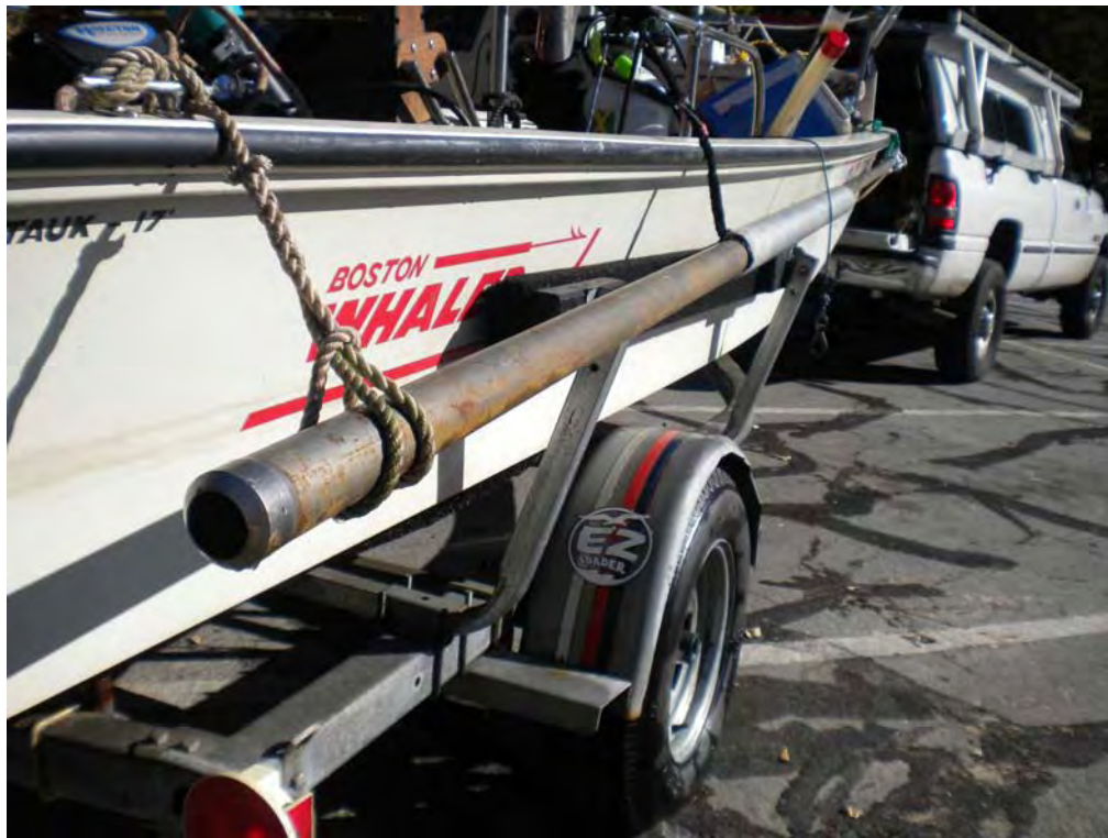
Photo 3: Modified Geoprobe® sludge soil sampler with underwater slide hammer mounted on boat.
