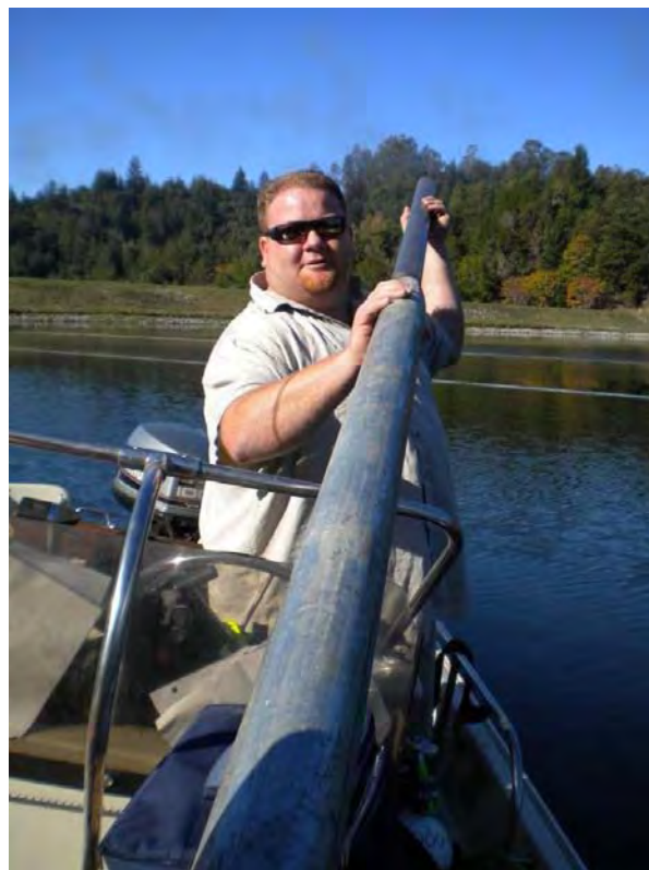
Photo 4: Modified Geoprobe® sludge soil sampler with underwater slide hammer ready to deploy.
