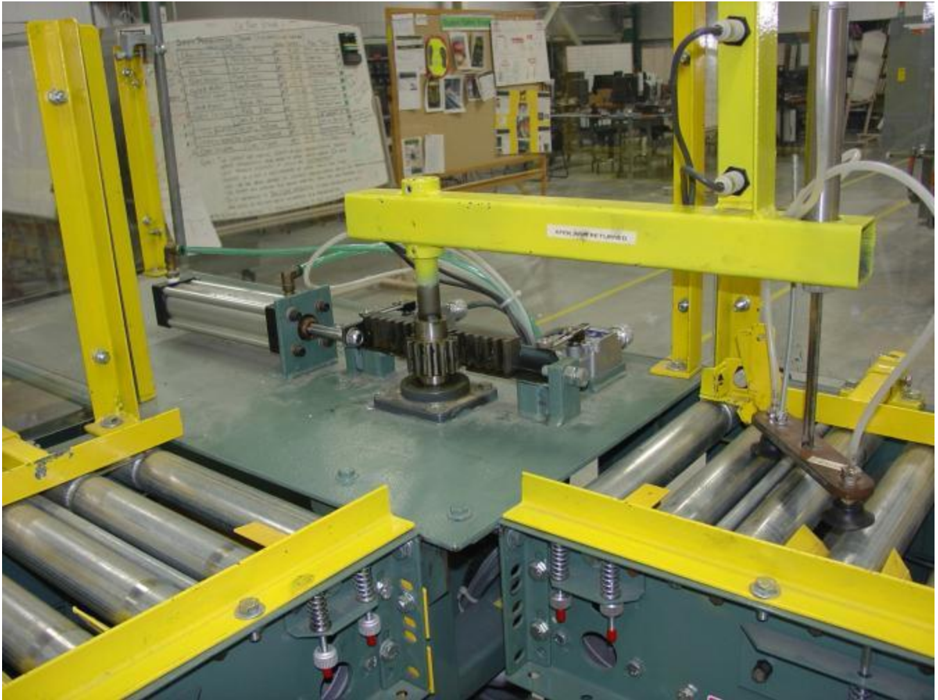
Conveyor Pick and Place (90 degree turn)
