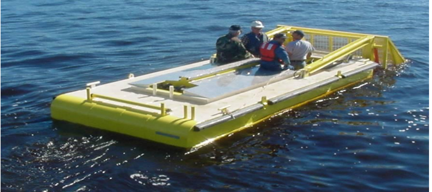
Vessel from rear showing cable guides & rear roller (below)
